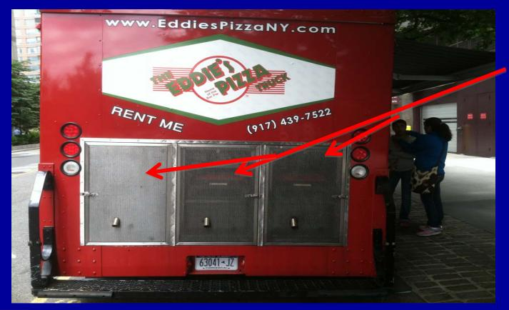
Three 4500 watt gasoline powered generators
